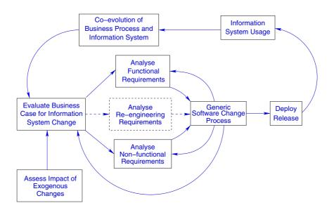
Figure 2. Software process model, Stereotype 2-high propensity for evolution.
