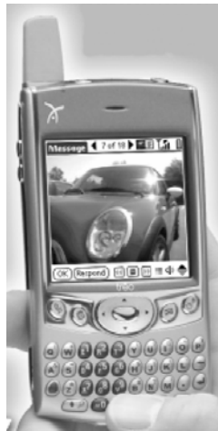
Fig. 7. PDA fashioned like Mobile Phone and including QWERTY keyboard
